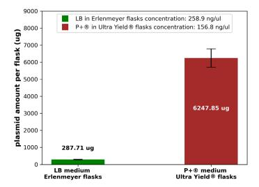
Figure 3a: Average total amount of purified plasmid (in µg) calculated per shake flasks used. Standard cultivation in 250 mL Erlenmeyer flask with a total filling capacity of 10% in green (left), Ultra Yield<sup>®</sup> flask with 250 mL flask with total filling capacity of 40% in brown (right). Flasks were cultivated at 350 min <sup>-1</sup>.
