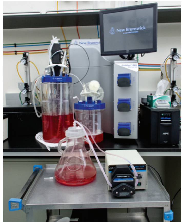
Transfer from flask to bioreactor with pump
