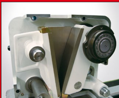
View of the grinding chamber with the housing removed
